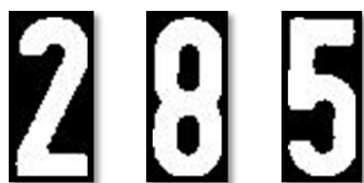
Figure 21. An example of the segmentation phase result.
