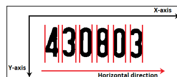
Figure 7. An illustration of the vertical projection. As a result, we expect to obtain a set of images, each of which containing one of the characters and ready for the next phase (the recognition phases).
