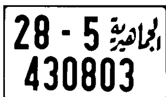
Figure 18. Result of binarizing the grayscale image.
