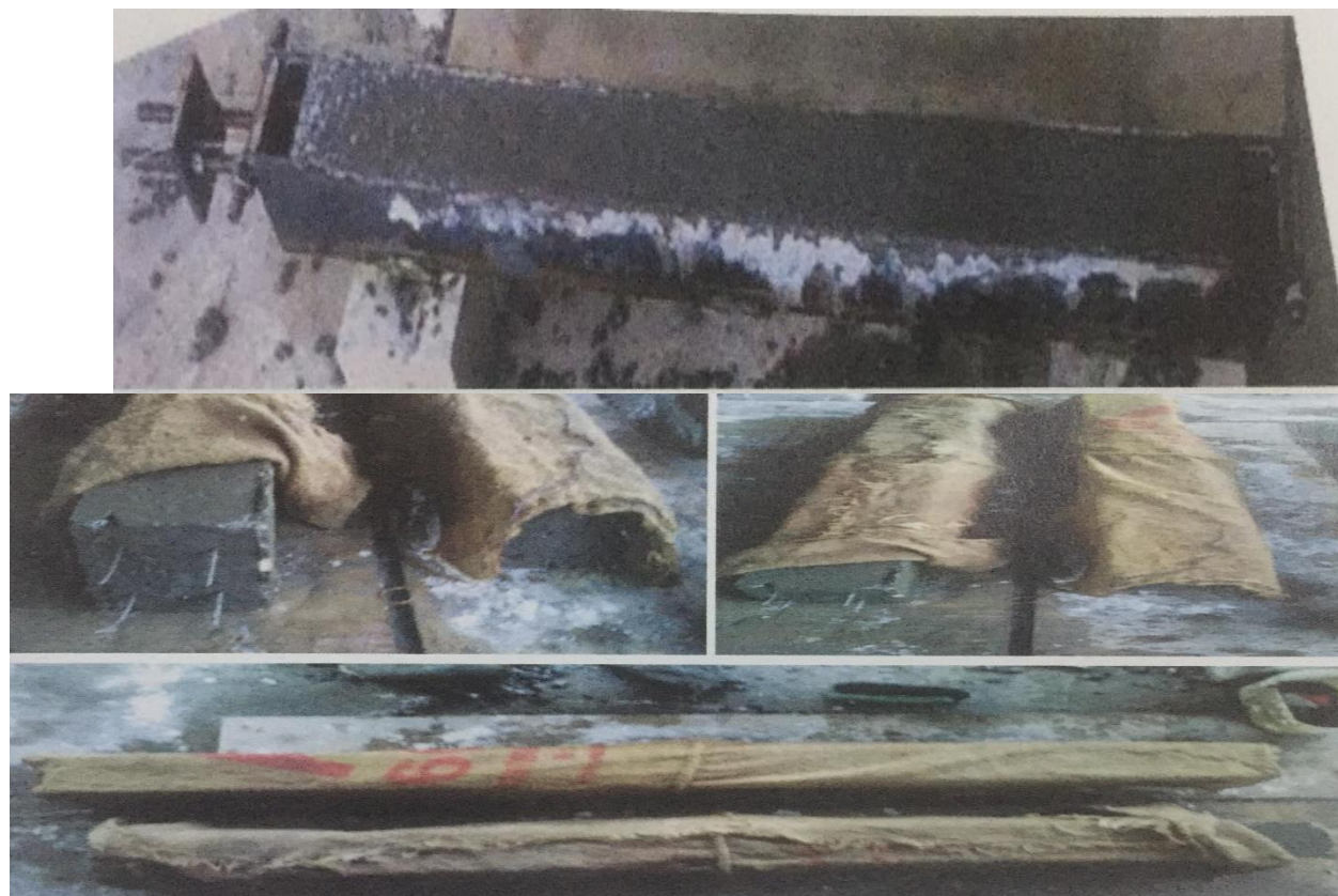
Figure 5 Casting of specimens and curing concrete
