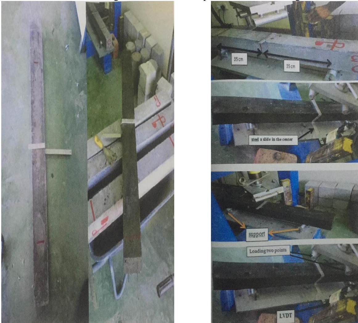
Figure 6 Steel a slide in the center of the prism to calculate the deflection during the test
