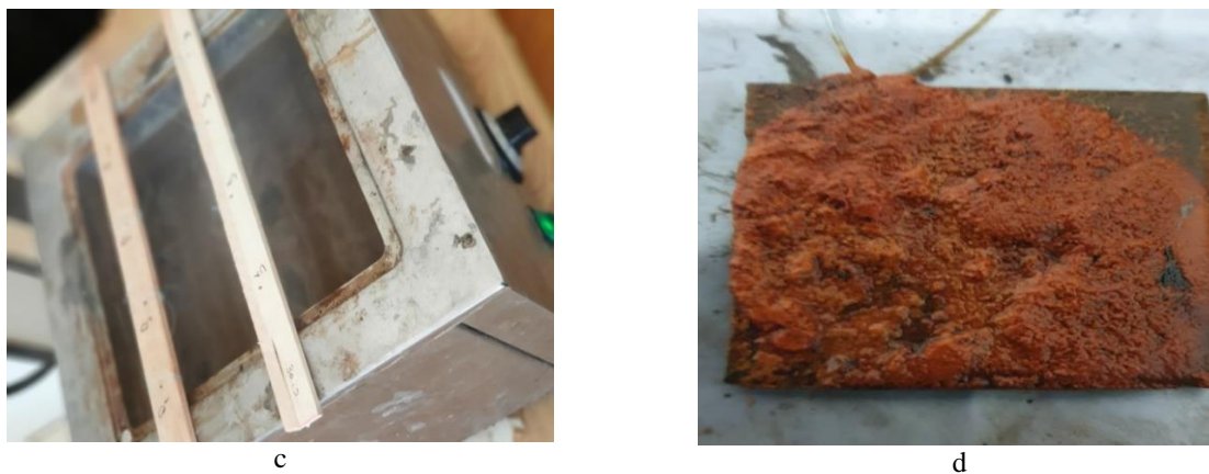
Figure 1: Representations of (a) a finished sample, (b) suspension of samples in aerated water, (c) heating of samples and (d) a sample after exposure time
