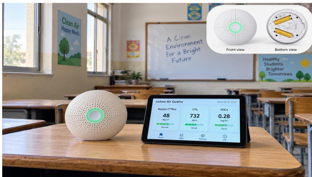
Figure 2. Indoor Air Quality Monitoring Device Installed in a Primary School Classroom for Measuring Radon, CO 2 , and VOCs.
