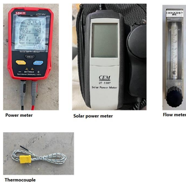
Figure 4. Experimental Measuring Instruments for PV Performance Evaluation.
