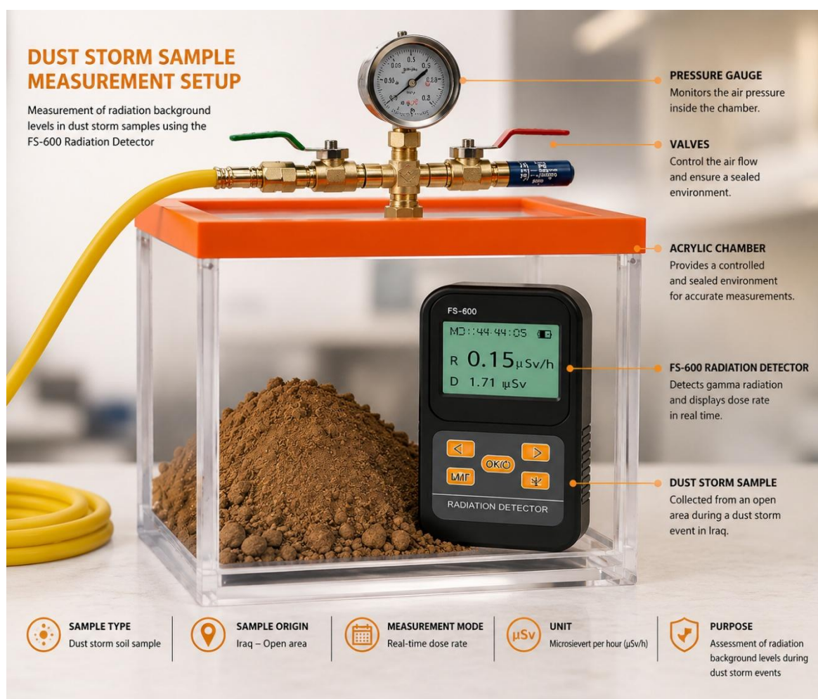
Figure 1. Experimental Arrangement Used for the Determination of Radiation Background Levels Resulting from Dust Storms in Iraq Using the FS-600 Radiation Detector
