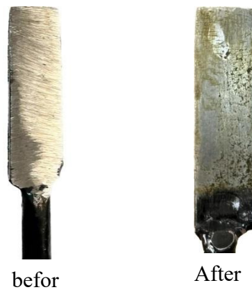
Figure 7: sample of mild steel befor immersion in sea water
