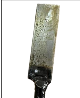
Figure 4: Mild steel after corrosion
