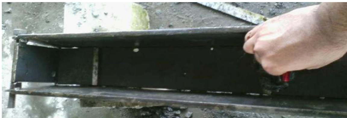
Figure 3.6: Grease was applied to the prism
