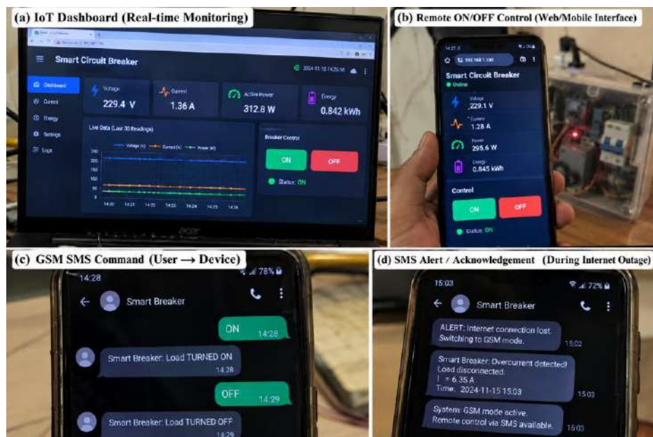
Fig. 6. Experimental IoT and GSM/SMS interface used during testing: (a) real-time monitoring of voltage, current, active power, and energy; (b) remote ON/OFF control; (c) GSM SMS command and acknowledgement; and (d) GSM fallback alert and acknowledgement during an Internet outage.
