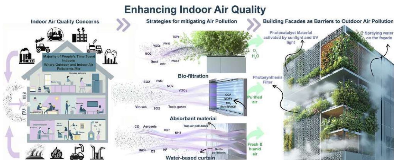
Figure 8. Environmental adaptability and indoor air quality enhancement in residential environments, illustrating how architectural elements, bio-filtration systems, absorbent materials, and responsive façade design strategies contribute to reducing indoor pollution and improving overall indoor environmental quality. Source: Jarrahi, A., Aflaki, A., Khakpour, M., & Esfandiari, M. (2024).
